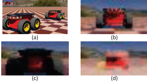
Fig. 5. (a) Webots simulation for case study, where ego vehicle (left) follows reference vehicle (right); (b) An example image captured by ego vehicle; (c) Lower bound of DNN input space; (d) Upper bound of DNN input space.
